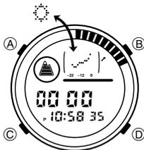
Auto Display automatically switches between the Barometer Mode's weather graphic and the barometric pressure graph. Note that you cannot use any of the watch's other functions while Auto Display is turned on.
