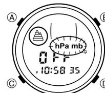
**Calibrating the Barometric Pressure Sensor**
