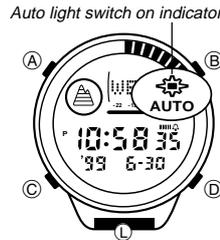
The backlight uses an EL (electro-luminescent) panel that causes the entire display to glow for easy reading in the dark. The watch's auto light switch automatically turns on the backlight when you angle the watch towards your face.
