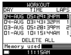
The Memory Used bar at the bottom of the screen indicates how much of the workout memory is used. You can store up to 20 workouts on the Global Trainer™ Bodylink® System watch, and the total number of laps in these workouts cannot exceed 1000.
