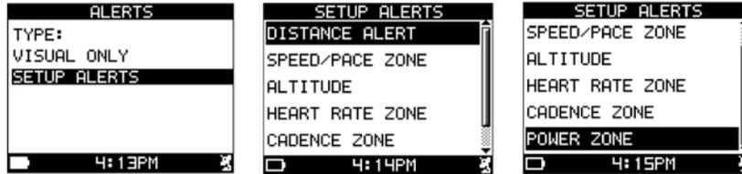
You can set minimum and maximum values for SPEED, HEART RATE, CADENCE, AND POWER. These values define the target zone for the setting. If the watch detects a value outside of this zone, the alert is triggered.
