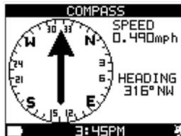
An arrow points to the 12 o'clock position while the compass ring spins around indicating the direction you are moving. Your current speed and your current heading (in direction and degrees) are listed to the right of the compass.
