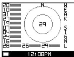
Press ▼ to highlight SATELLITE VIEW, then press ↵ to view a graphical representation of the satellites the Global Trainer™ Bodylink® System watch is fixed upon.
